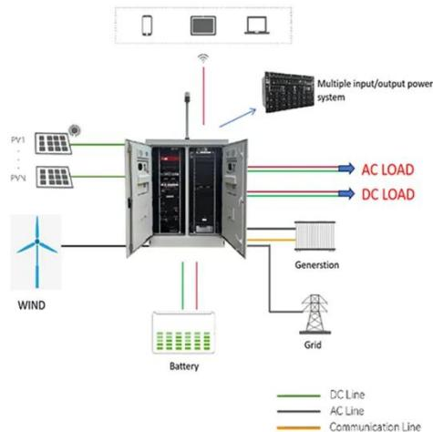
energy storage converter (PCS), 1260KWh battery system, one set of energy management system (EMS), isolation ...
