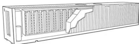
A flow battery is an electrochemical energy storage system that stores energy in liquid electrolyte solutions. Unlike conventional batteries, which store energy in solid electrodes, flow batteries ...
