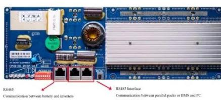
RS485 Communication between battery and inverters
